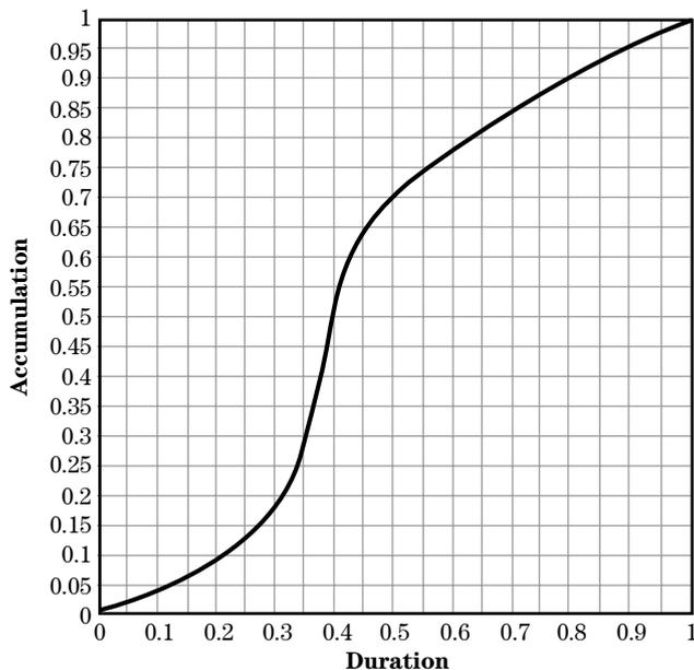
**(b) Development of the stability design hydrograph (SDH) and the freeboard hydrograph (FBH)**
